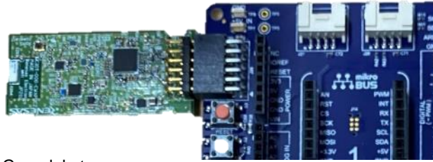
Connect Sub-G module to PMOD1 connector
