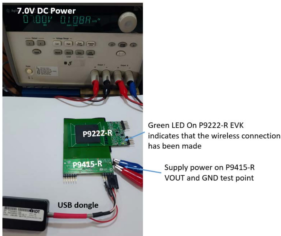
Figure 3. Evaluation Kit Connections for Rx Mode Test (2)
