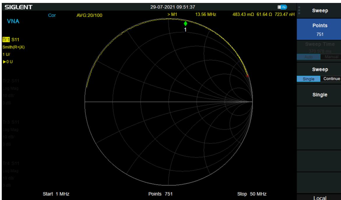
Figure 10. Smith Chart – Loop Antenna Measurement with VNA
