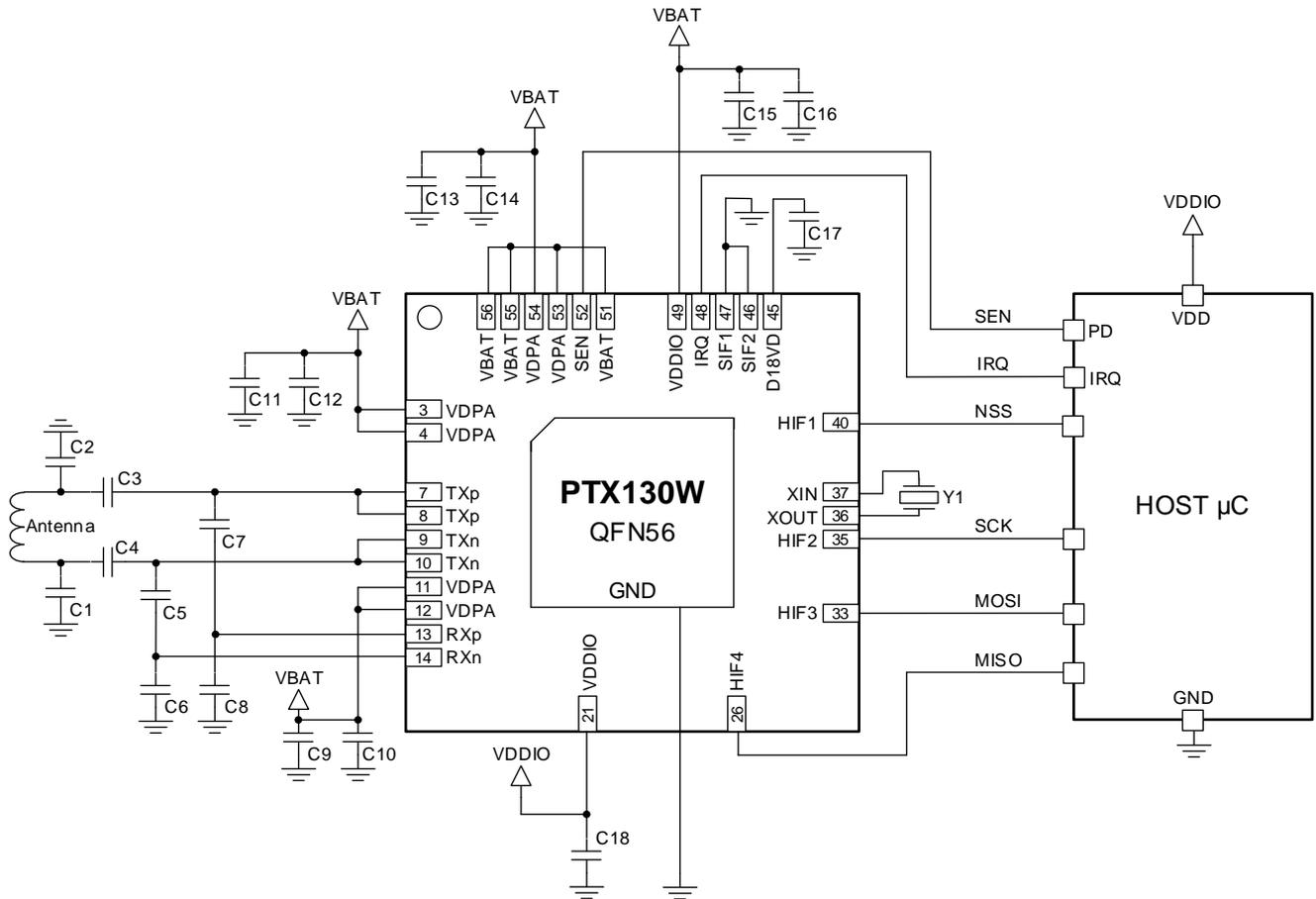
Figure 2. Typical PTX130W Application Schematic
