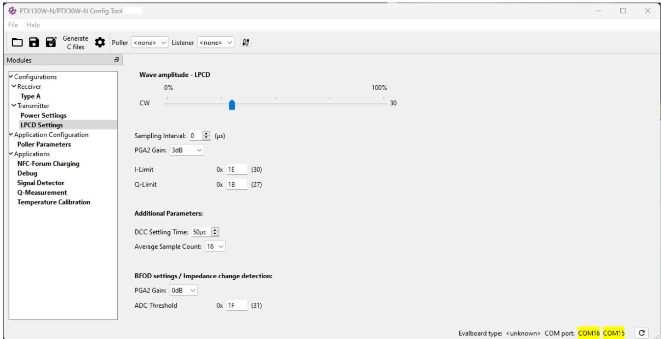
Figure 16. Config Tool LPCD Settings Window
