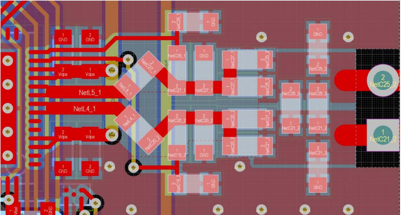
However, component tolerances and manufacturing differences can impact that effect. To that end, the matching network should also be created in a way that allows unwanted HF signal components to be dissipated to GND. A recommended matching network configuration to start with is shown in Figure 4.
