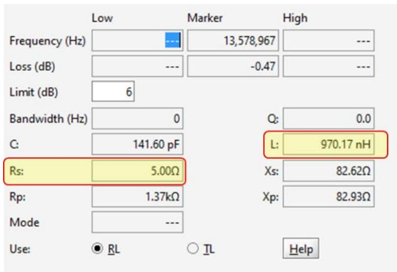
Based on this measurement, it is possible to extrapolate the electrical parameters of the antenna.
