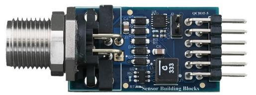
Figure 1. QCIOT-5 IO-Link Device Transceiver Board Image
