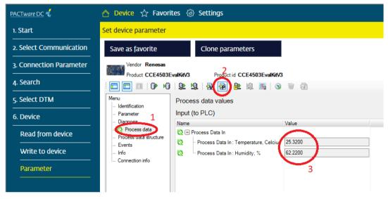
Figure 23. Cyclic Reading of the Data Values
