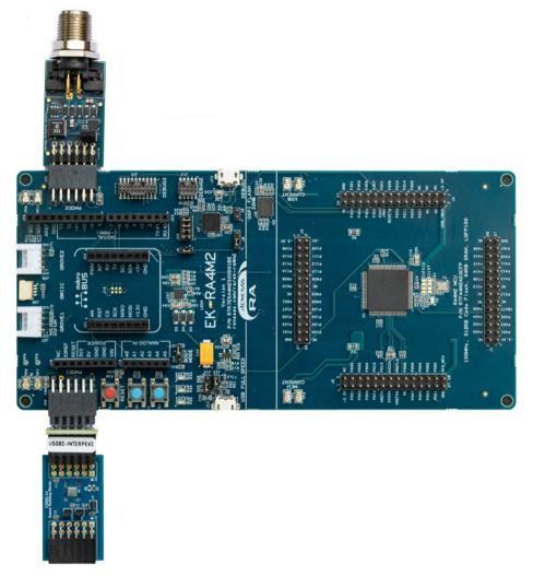
Figure 14. QCIOT-5 IO-Link Device Pmod Test Setup
