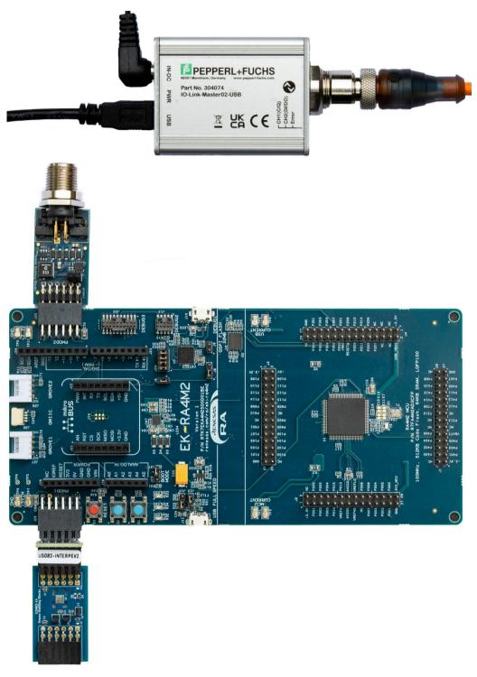
Figure 3. QCIOT-5 IO-Link Device CCE4503 Test Setup
