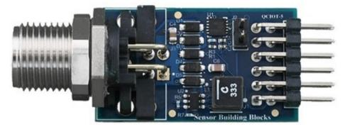
Figure 4. QCIOT-5 IO-Link Device Transceiver Board (Top)
