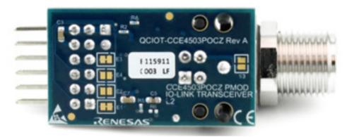
Figure 5. QCIOT-5 IO-Link Device Transceiver Board (Bottom)
