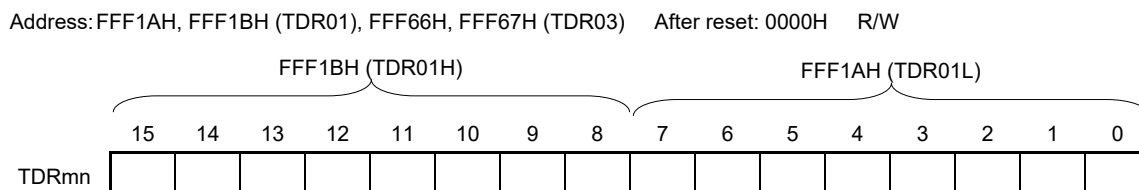
Figure 6-8. Format of Timer Data Register mn (TDRmn) (n = 1, 3)
