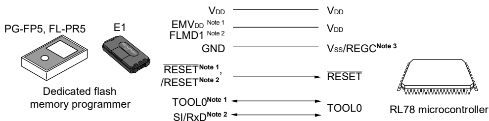
Figure 28-2. Communication with Dedicated Flash Memory Programmer
