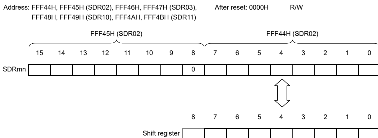
Figure 14 - 4 Format of Serial data register mn (SDRmn) (mn = 02, 03, 10, 11)
