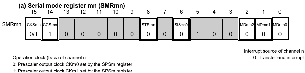
Figure 14-85 Example of Contents of Registers for Slave Reception of Slave Select Input Function (CSI00) (1/2)
