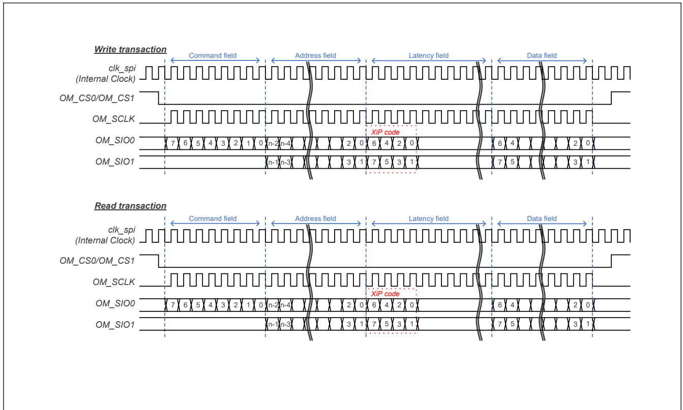
Figure 35.4 1S-2S-2S timing-chart
