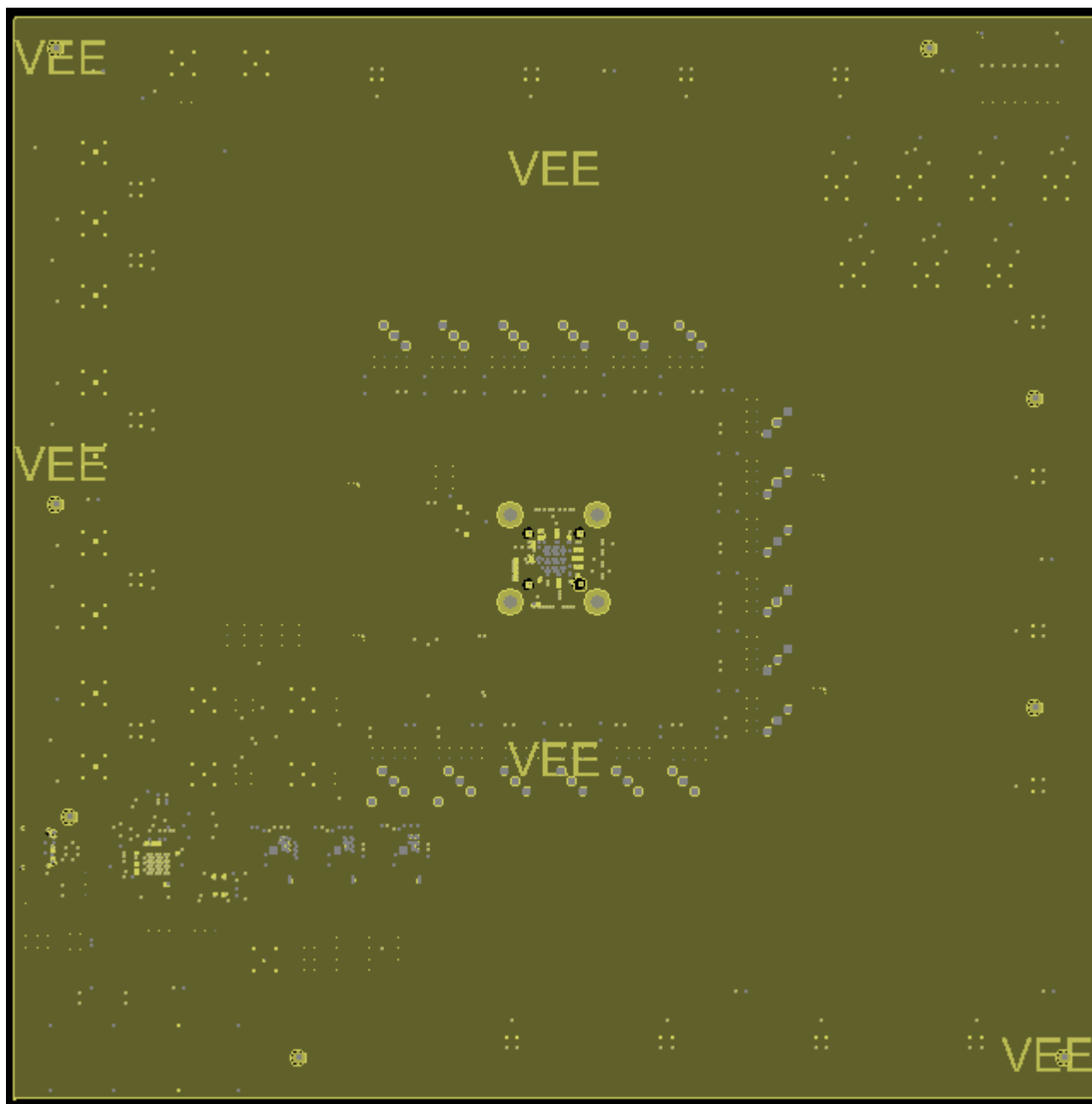
Figure 35. Layer 4-VEE Plane
