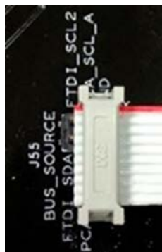
Figure 9. Aardvark Adapter Connection to J55
