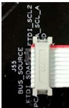
Figure 9. Aardvark Adapter Connection to J55
