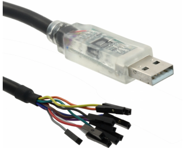
Figure 6. FTDI Dongle: USB Type-A at PC end and 10 Free-wires at the other end
