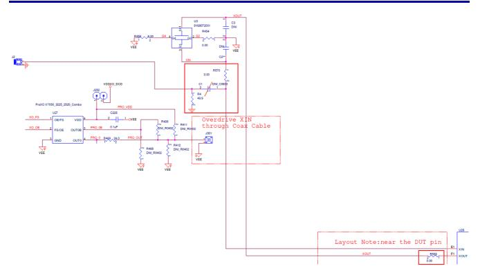
**Figure 9. Crystal Mount Schematic**
