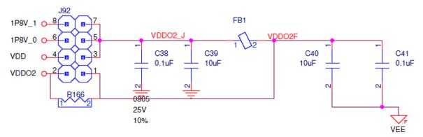
Figure 7. VDD Jumper Bypass Schematic
