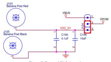
Figure 5. External 5V Schematic
