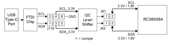
Figure 16. Communication Setup for I<sup>2</sup>C Mode
