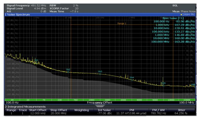
Figure 32. Phase Noise 491.52MHz Output Synthesizer Mode
