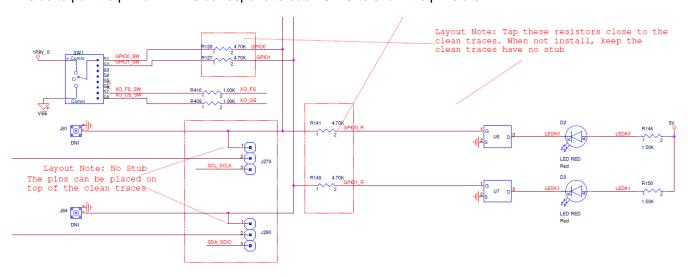
Figure 22. GPIO Schematic and EVB DIP Switches
