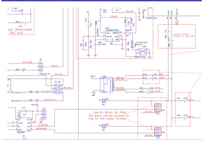
Figure 21. EEPROM Connection Jumpers for RC38208A GPIO
