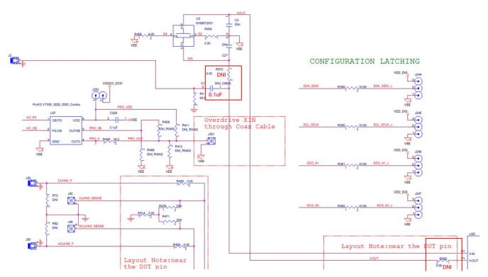
Figure 8. XIN Pin Overdrive Schematic
