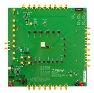
Figure 30. RC38208A Evaluation Board (Top)
