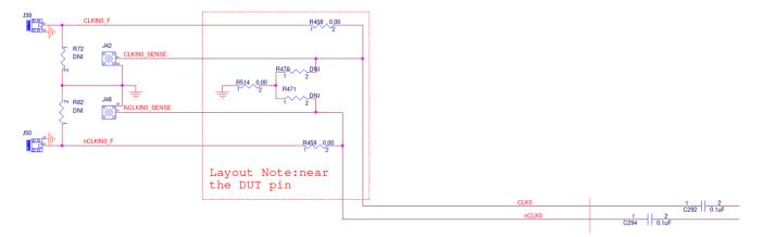
Figure 13. Input Clock with Sense Schematic
