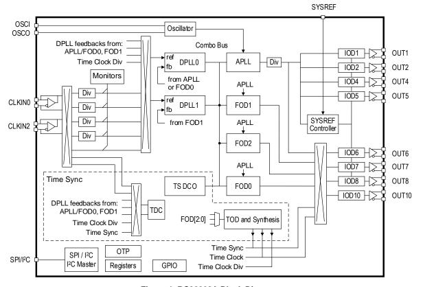
Figure 1. RC38208A Block Diagram
