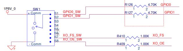
Figure 12. XO\_OE and XO\_FS Pins DIP Switch Schematic
