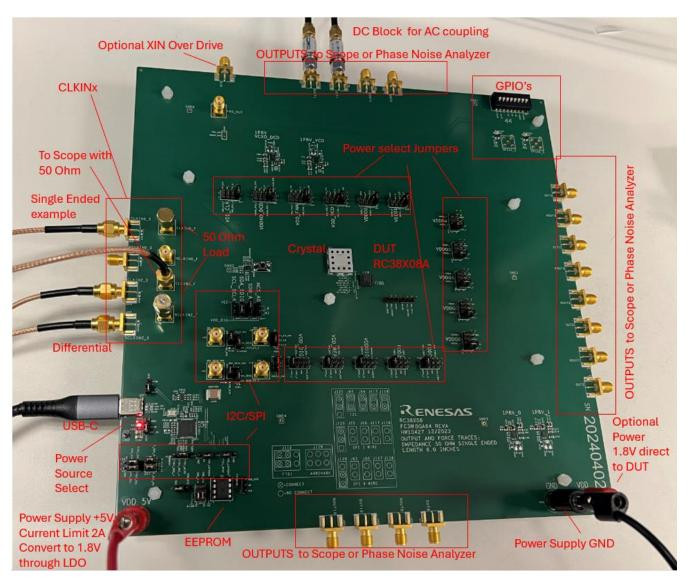
Figure 2. Evaluation Board - General Setup
