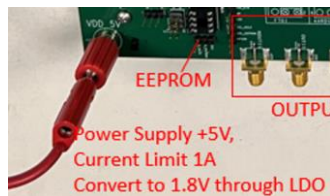
Figure 4. External 5V Board Input
