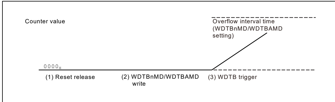
Figure 31.4 Timing Diagram of WDTB Start in Software Trigger Start Mode
