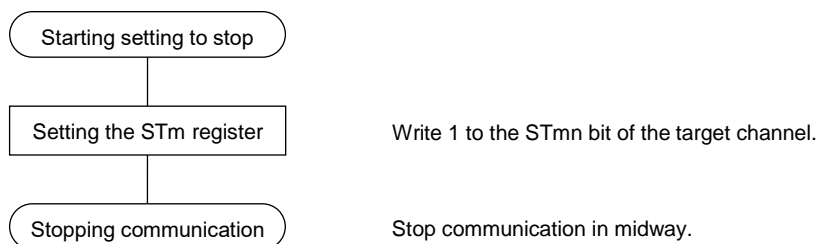
Figure 15-86. Procedure for Stopping Master Reception
