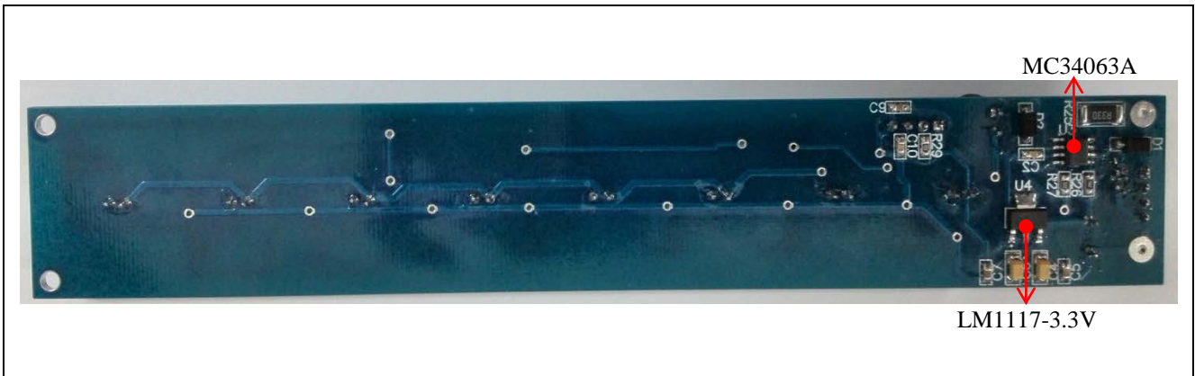
Figure 2.2 Bottom View of the Safety Light Curtain Transmitter
