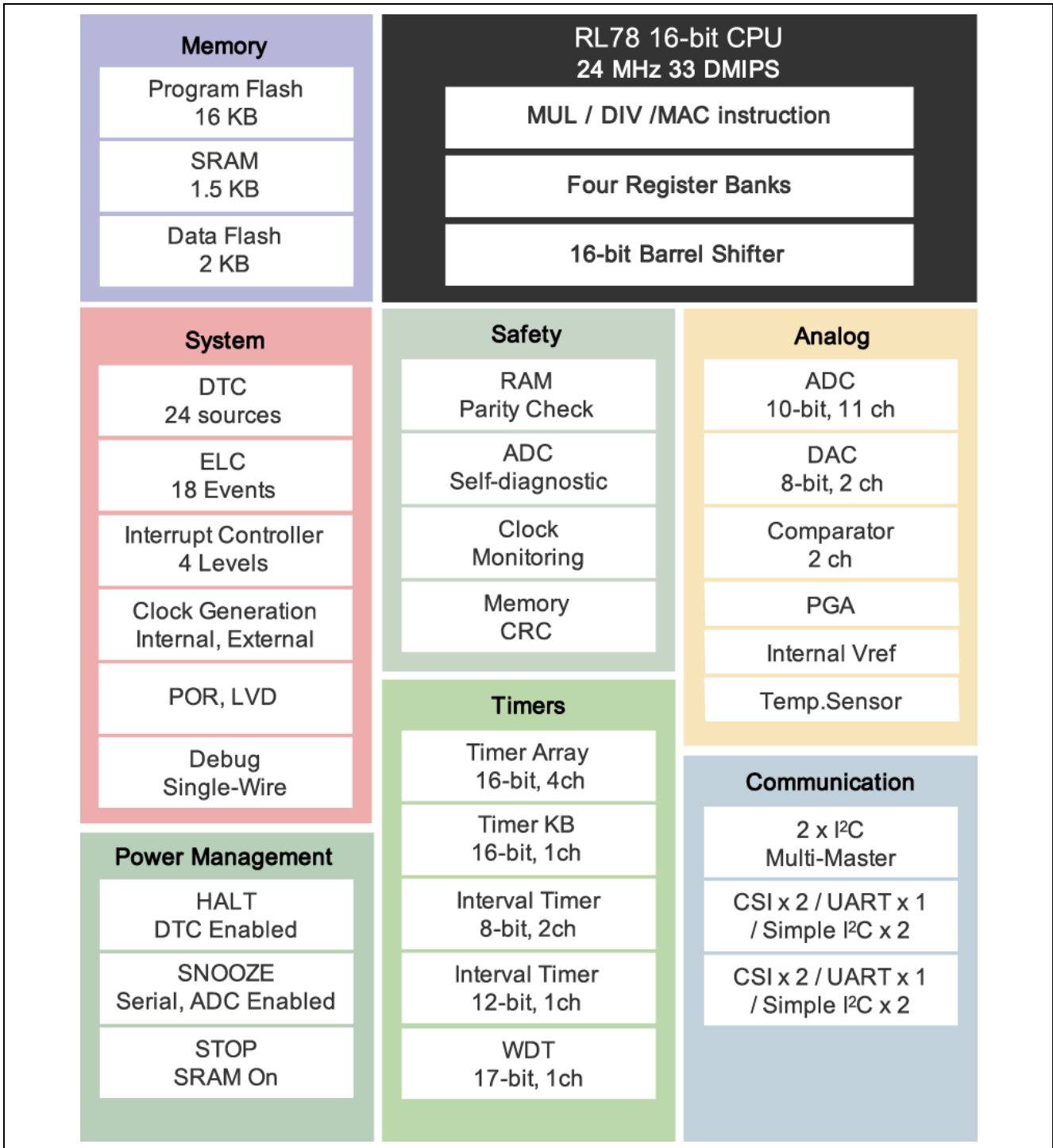
Figure 2.1 RL78/G11 (20-pin products) Block Diagram
