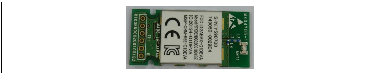
Figure 2.3 Circuit Board of RL78/G1D Module
