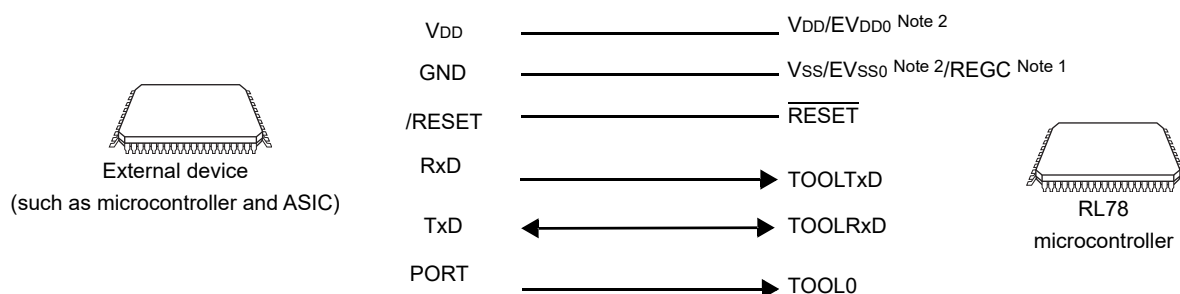
Figure 33 - 4 Communication with External Device
