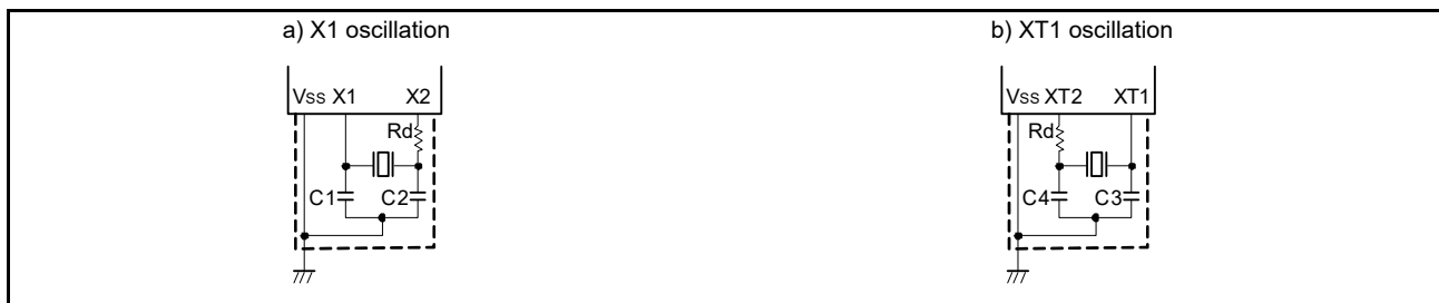
Figure 9 - 28 Examples of External Circuits
