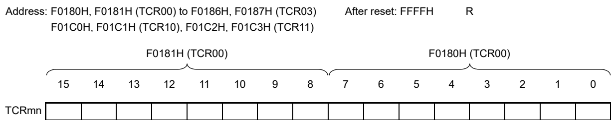
Figure 6 - 9 Format of Timer counter register mn (TCRmn)
