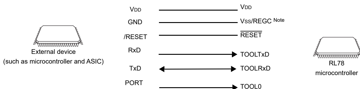
Figure 30 - 4 Communication with External Device
