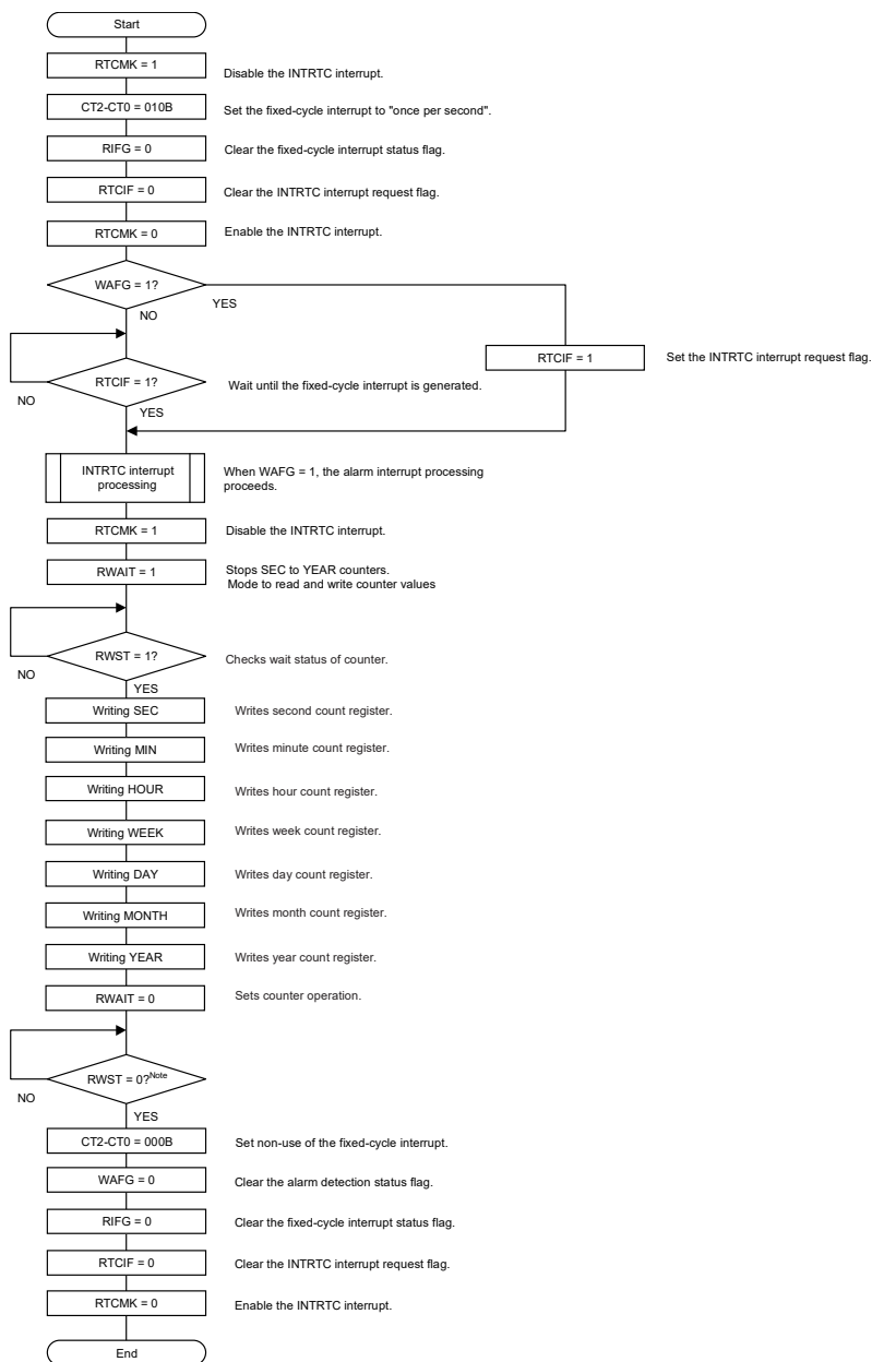
Figure 7-24. Procedure for Writing Real-time Clock (When the Alarm Interrupt is in Use)
