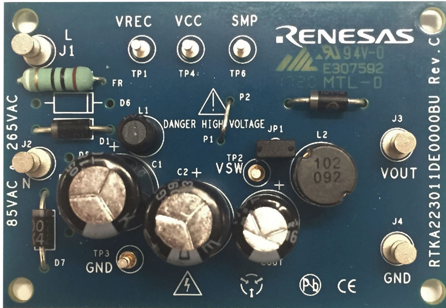
Figure 2. RTKA223011DE0000BU Evaluation Board (Top)
