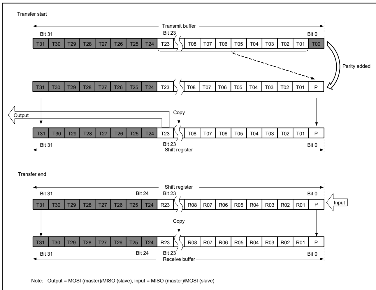
Figure 30.19 MSB First Transfer (24-Bit Data, Parity Enabled)
