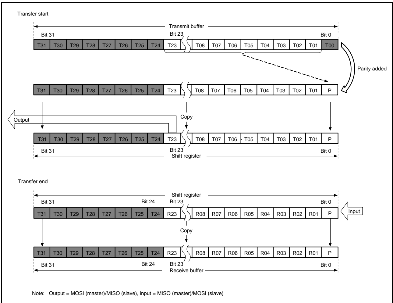
Figure 34.19 MSB First Transfer (24-Bit Data, Parity Enabled)
