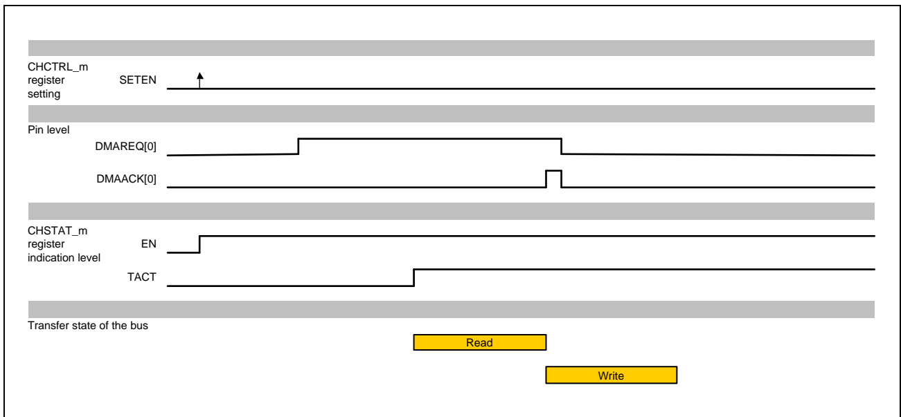
Figure 18.6-26 DMAC State Example 1 (Hardware Request)
