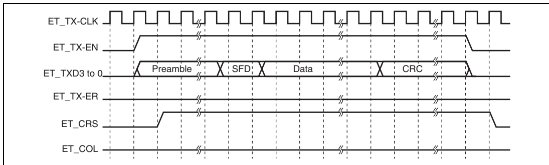
Figure 24.15 MII Frame Transmit Timing (Normal Transmission)
