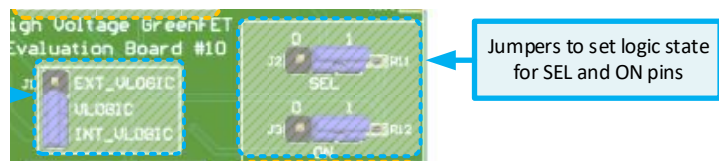
Figure 10. SEL/ON Logic State Selection
