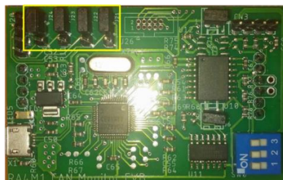
Figure 3-2 Program Development/Debugging Using JLINK on RA4M1 Monitor EVB
