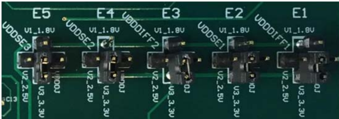
Figure 3. Jumper Configuration for On-board Voltage Regulators
