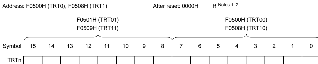
Figure 11 - 3 Format of 8-bit interval timer counter register n (TRTn)
