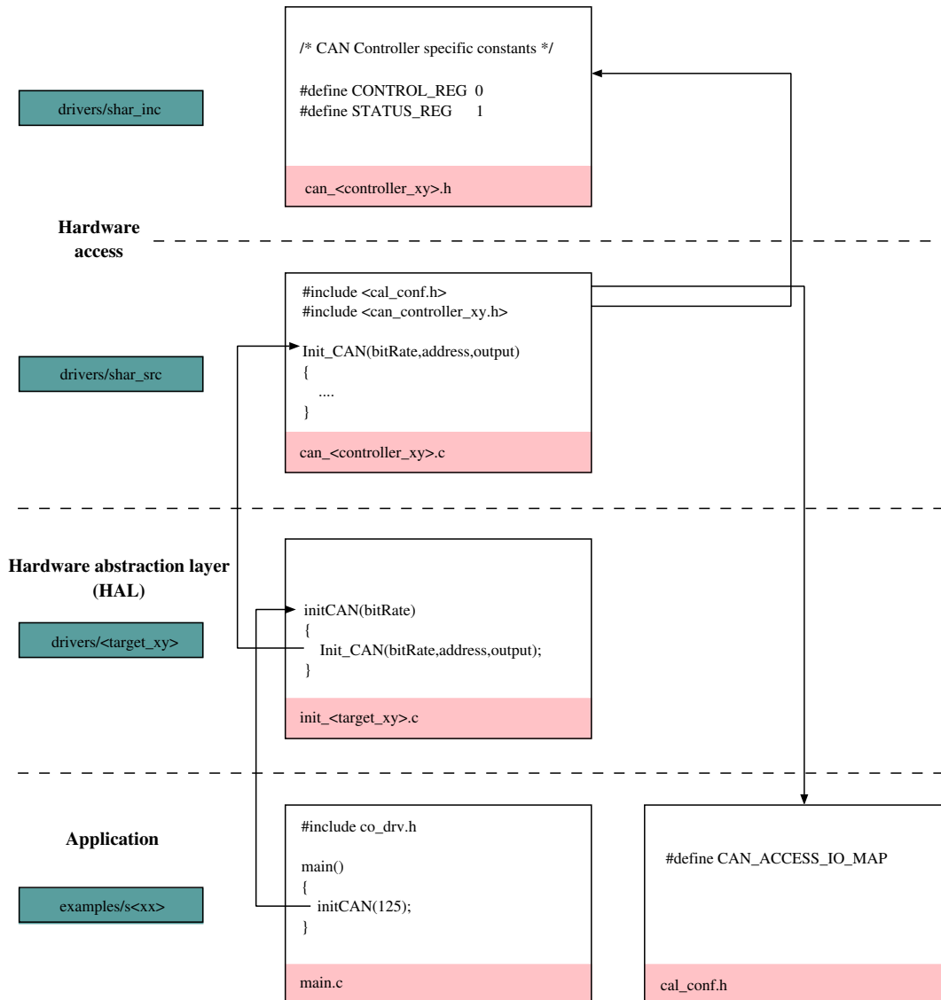
Figure 43, Hardware Abstraction Layer Realization
