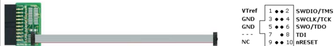
Figure 28: J-Link 9-pin Cortex-M adapter
