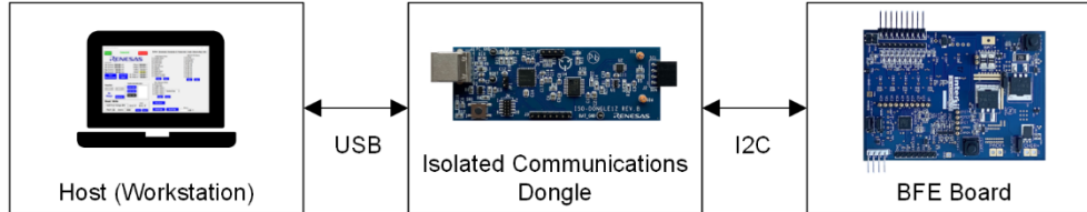
Figure 1. GUI, Communications Dongle and Battery Front End Connection
