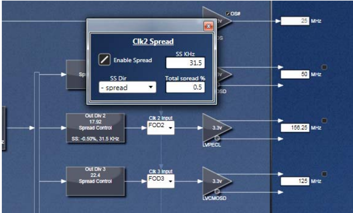
Figure 10. Spread Spectrum Control Window
