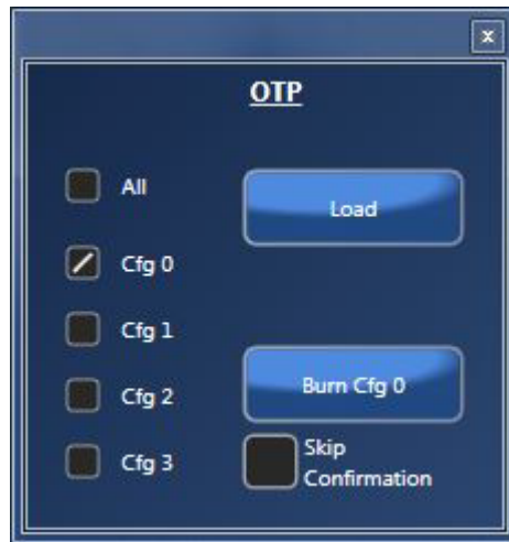
Figure 17. OTP Programming within Timing Commander GUI
