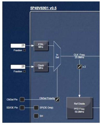
**5. Input Frequency Fraction box** – - Input clock can be entered as a fraction if fraction box is checked and Fraction word is clicked as shown in figured 5c below. The calculation button will give the final frequency that will be entered in the input box. The fraction can be used for both Xtal and CLKin inputs.
