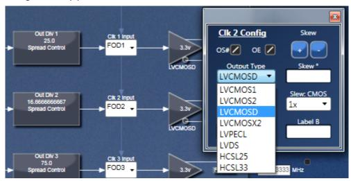
Clicking on the triangle box brings about output frequency configurations: Output type, Slew rate, Output voltage and Skew.
