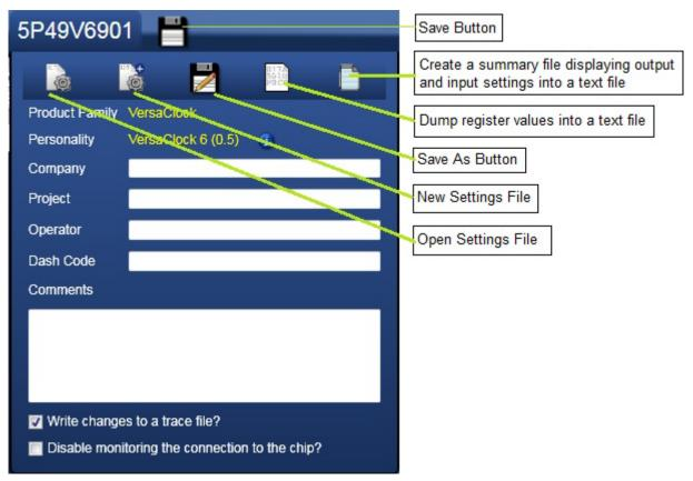
**8. Save the Settings File** – After the configuration is complete, click on the disk symbol at the upper left corner to save the setting file, as shown below.
