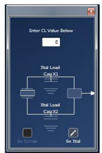
The max CL that can be created in the IC is 11.4pF. When entering a larger value, Timing Commander will display a window advising how much capacitance to add externally to each crystal pin to achieve the desired CL value (see Figure 6). TC is rounding the values to a integer value for the advisable external capacitors.
