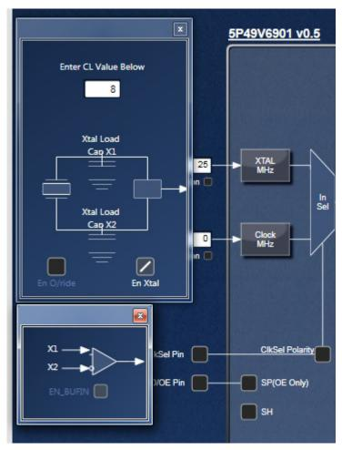
There are situations where both crystal and CLK are used as input sources. In this case, check both "En Xtal" and "EN\_BUFIN". Then use CLKSEL pin to select crystal or CLK source to be used as the input reference. The Truth Table is listed in table 1 below.
