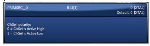
The CLKSelPol check box needs to be checked if using the CLK is selected as primary source and if CLK sel pin low like in Figure 5b. The timing commander will display the selected source based on the selection. The En\_Buff box will be then enabled.
