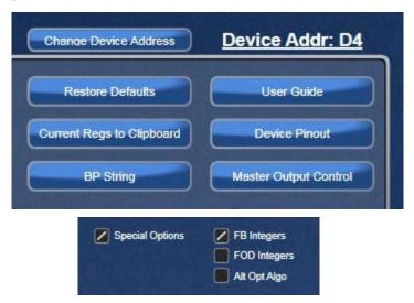
When connected to the device it is possible to change the I2C address by clicking on the **Change Device Address** button. This is permanent change that cannot be reversed.
