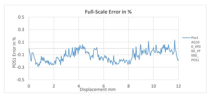
Figure 3. Accuracy with Linearization at 1mm Airgap (AG100)
