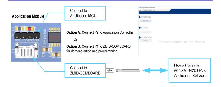
**Figure 1. Application Module Connections**
