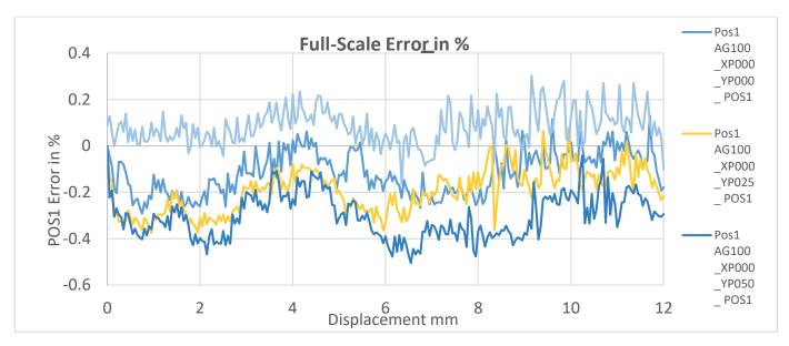
Figure 5. Accuracy with Linearization at 1mm Airgap and Effects of Displacement
