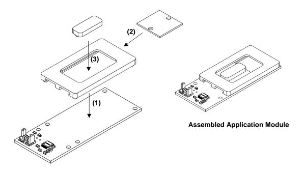
Figure 2. Target Holder Assembly
