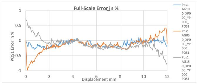
Note: AG050 = 0.5mm airgap; AG100 = 1mm airgap; and AG150 = 1.5mm.
