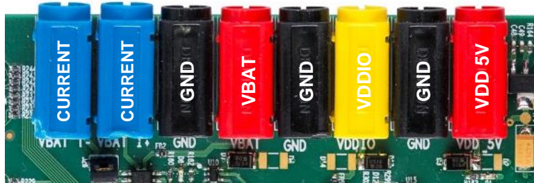
Figure 4: PLT Hardware Power Connections
