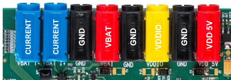
Figure 4: PLT Hardware Power Connections
