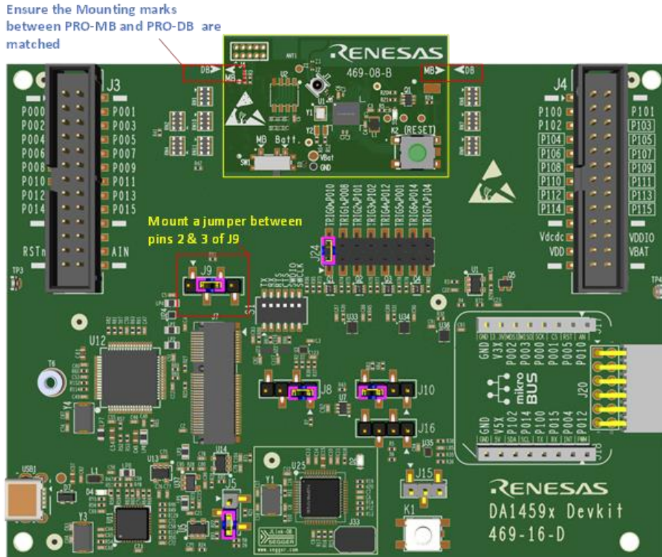
Figure 5. Hardware setup of DA1459x Pro-Devkit without PMM2
