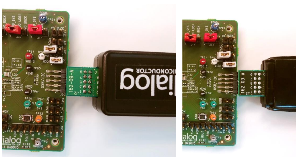
Figure 2: USB-I2C Module and VDDIO Connection
