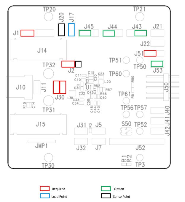
**Figure 1: Typical Jumper Positions and Connection Points**
