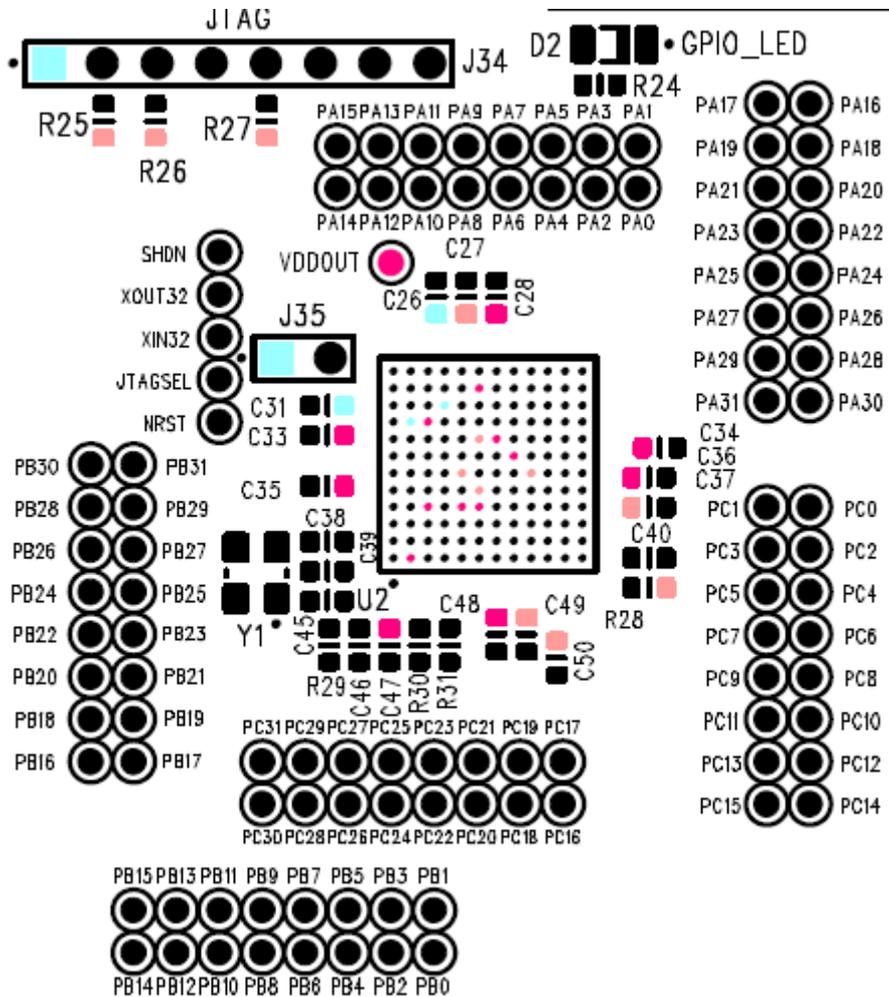
Figure 3: ATSAM3U  $\mu$ -Controller for USB-I2C bridge
