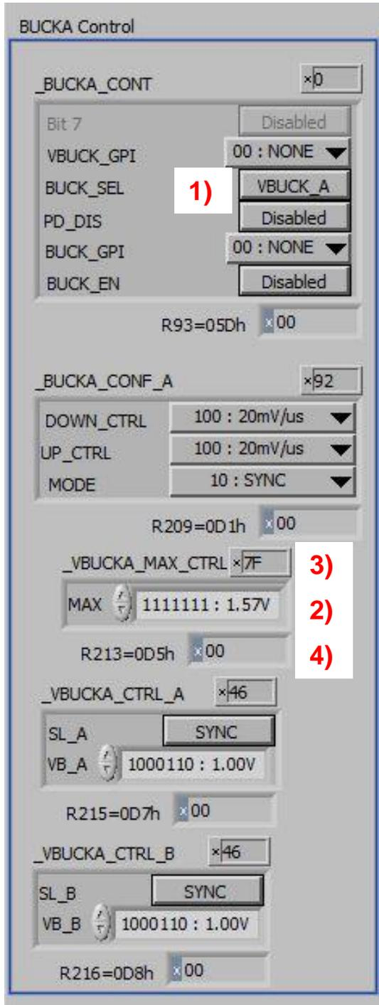
Changing a register control immediately sends the value to the selected register, and reads the value back again, comparing the result with the hex indicator. Note that all bits of the register are sent at once. Therefore this does not allow changing multiple bits simultaneously.
