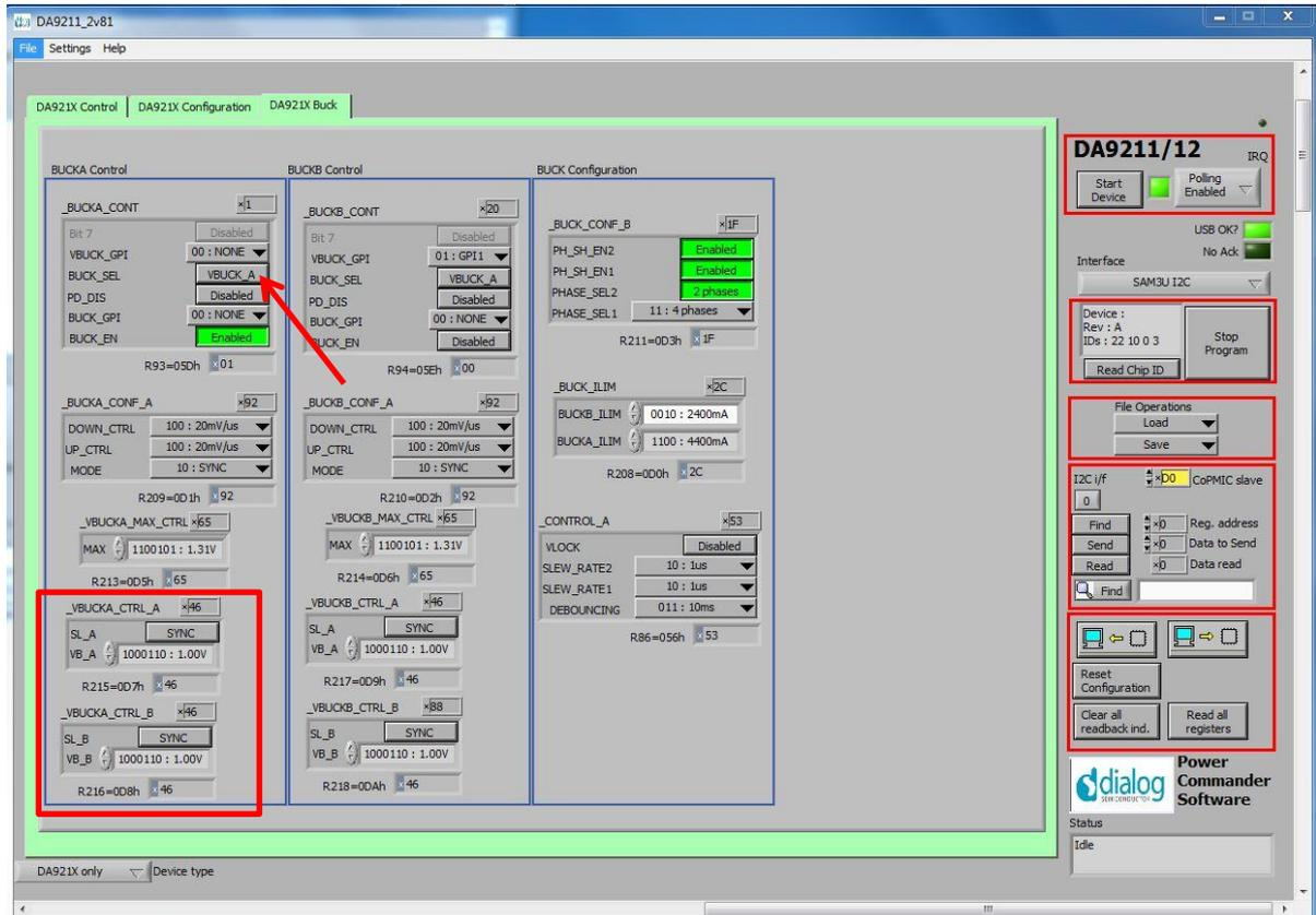
**Figure 15: Output voltage control of the buck**
