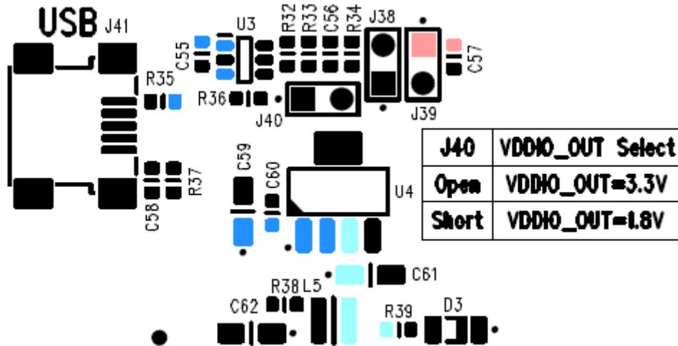
Figure 4: Mini USB input and internal rails generation
