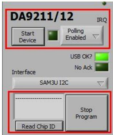
Press the Start Device button to correctly configure the software for stand alone operation. We are now able to control DA9212 in stand alone mode. In this mode DA9212 acknowledges all I2C commands, which does not always happen if DA9212 is in companion mode.
