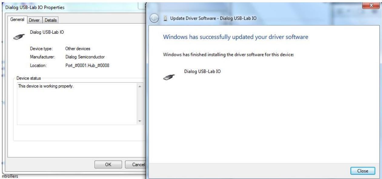
If installed correctly, Dialog USB Driver should be listed on Device Manager.
