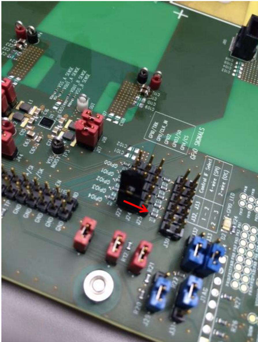
**Figure 17: Port control of the buck output voltage**
