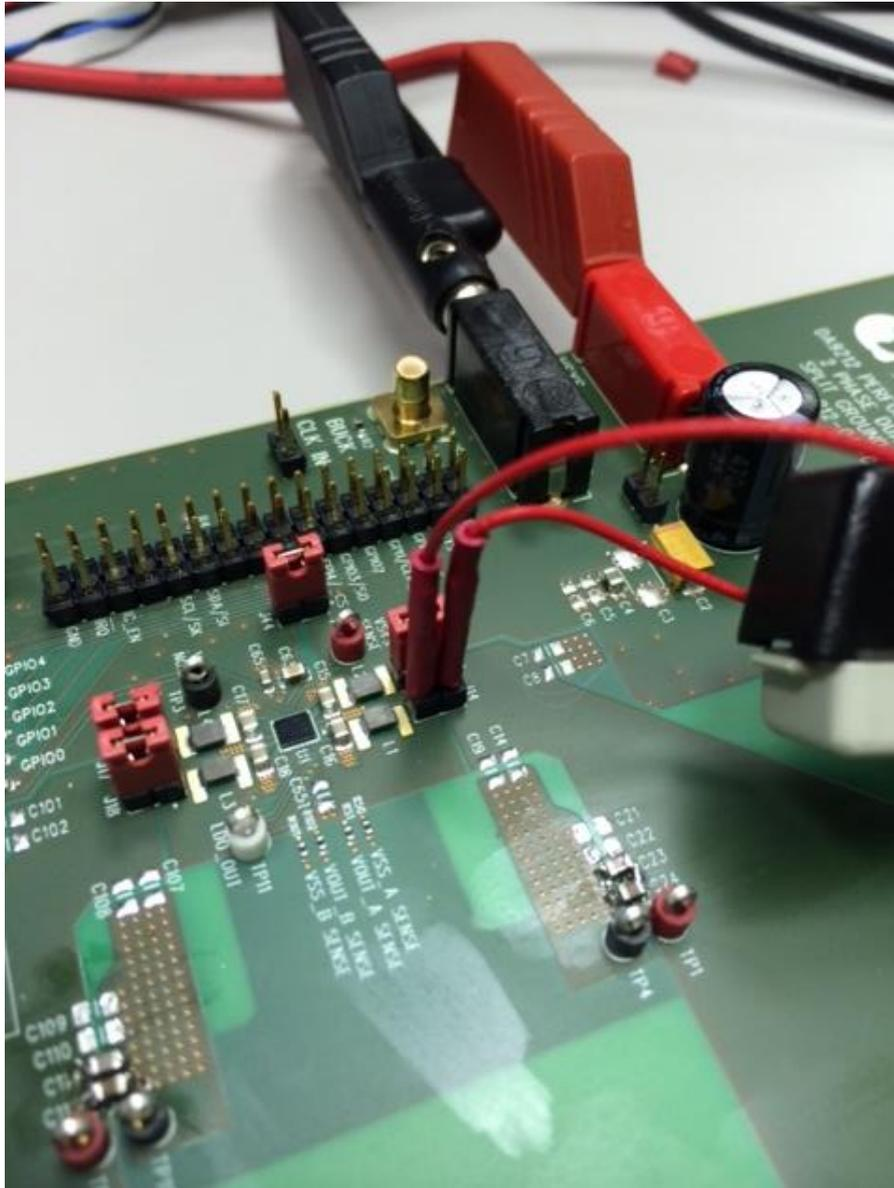
**Figure 12: Sensing the LX signals of buck A**
