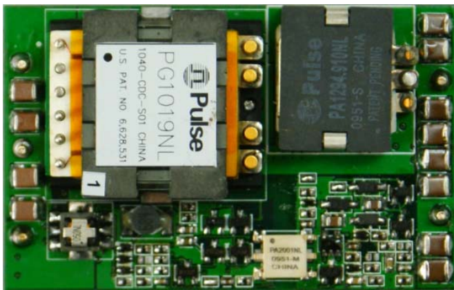
FIGURE 1. TOP VIEW OF ISL6726EVAL1Z (ACTUAL SIZE: 40x60x16mm)
