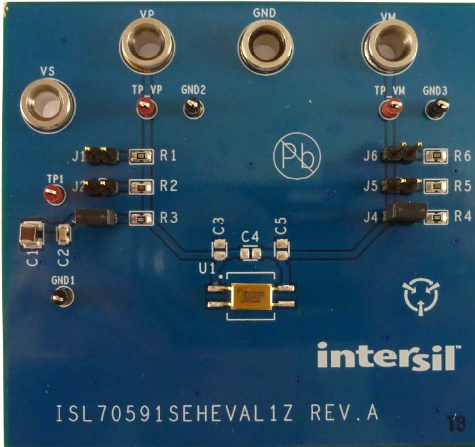
Figure 3. ISL70591SEHEVAL1Z Evaluation Board
