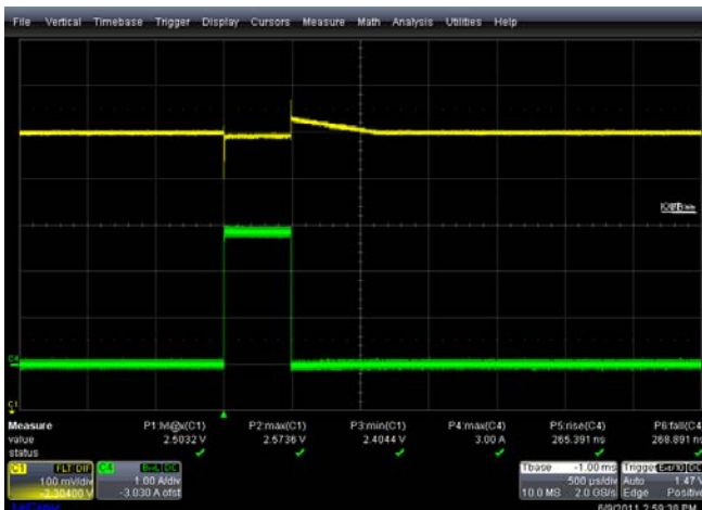
FIGURE 7. LOAD TRANSIENT, V_{IN} = 3.3V , V_{OUT} = 2.5V , C_{OUT} = 47\mu F 35mΩ
