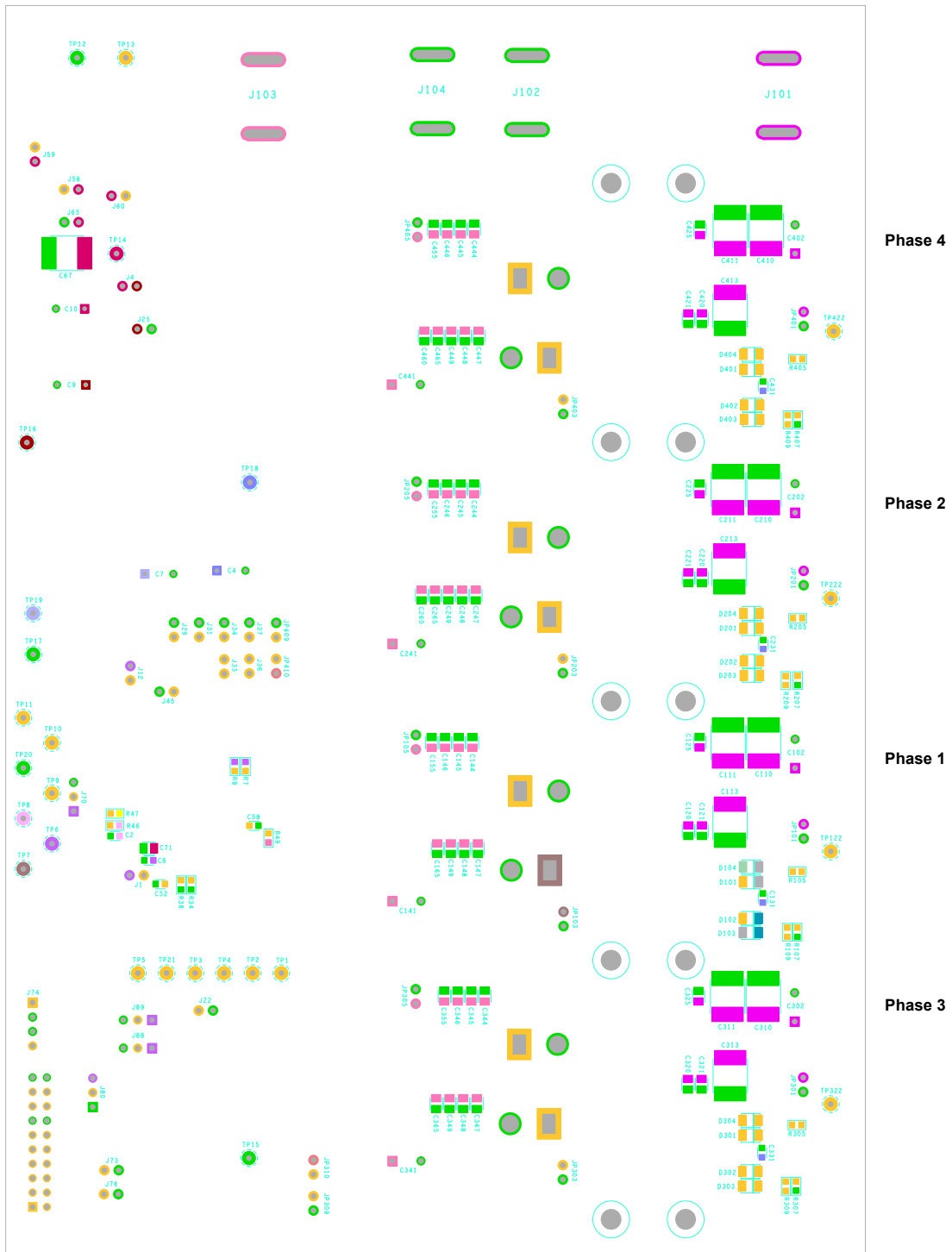
Figure 96. PCB – Silkscreen Bottom (Viewed from Bottom)
