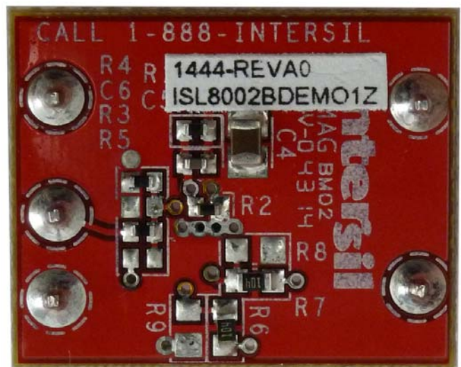
FIGURE 2. ISL8002BDEMO1Z BOTTOM SIDE
