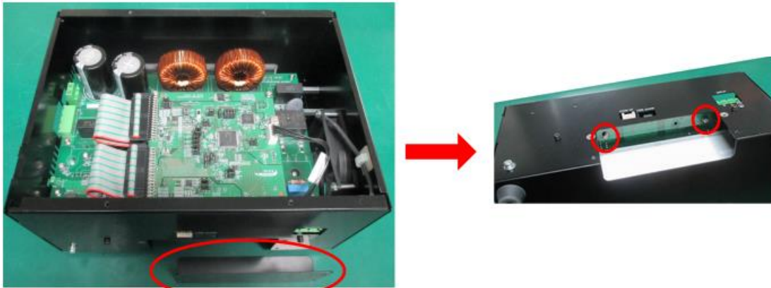
Fig. 3-3 Board Connection (CPU board : inverter board)
