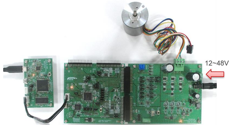
Figure 4-10 Power supply from DC jack
