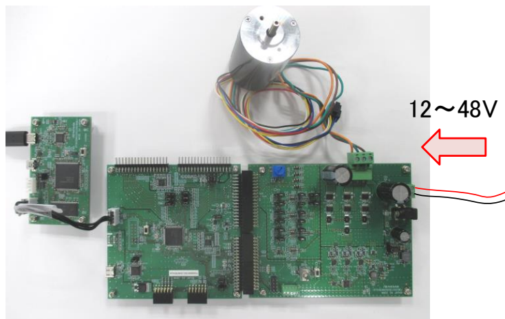
Figure 4-11 Power supply from terminal block
